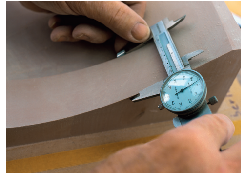
Achieve master models of high dimensional accuracy with SikaBlock® M600 N and SikaBlock® M700 N.
