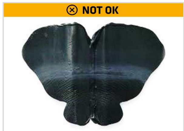
Figure 7: Unfold the foil - Negative test = inadequate mixing
