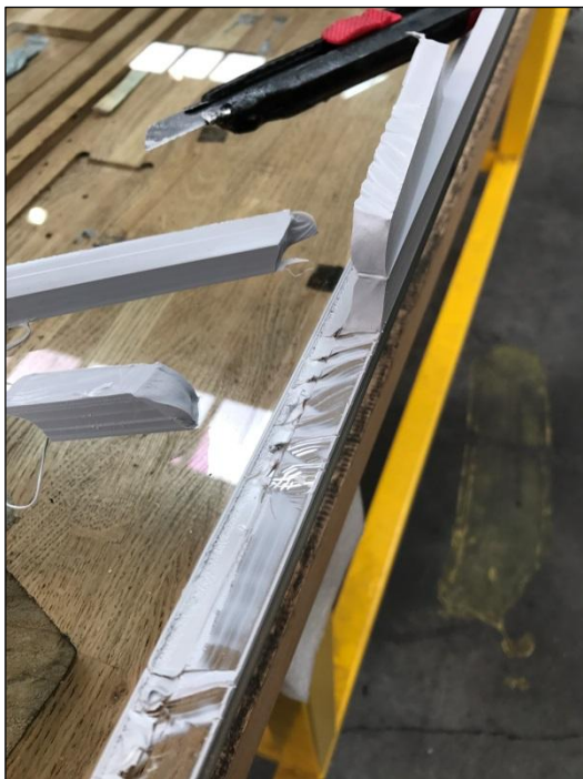
Figure 35: Good adhesion, deglazing test positive
