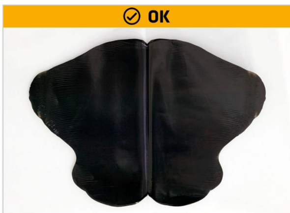
Figure 6: Unfold the foil - Positive test = ideal mixing
