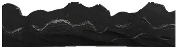
Figure 11: Severe white stripe in material, inhomogeneous mixing
