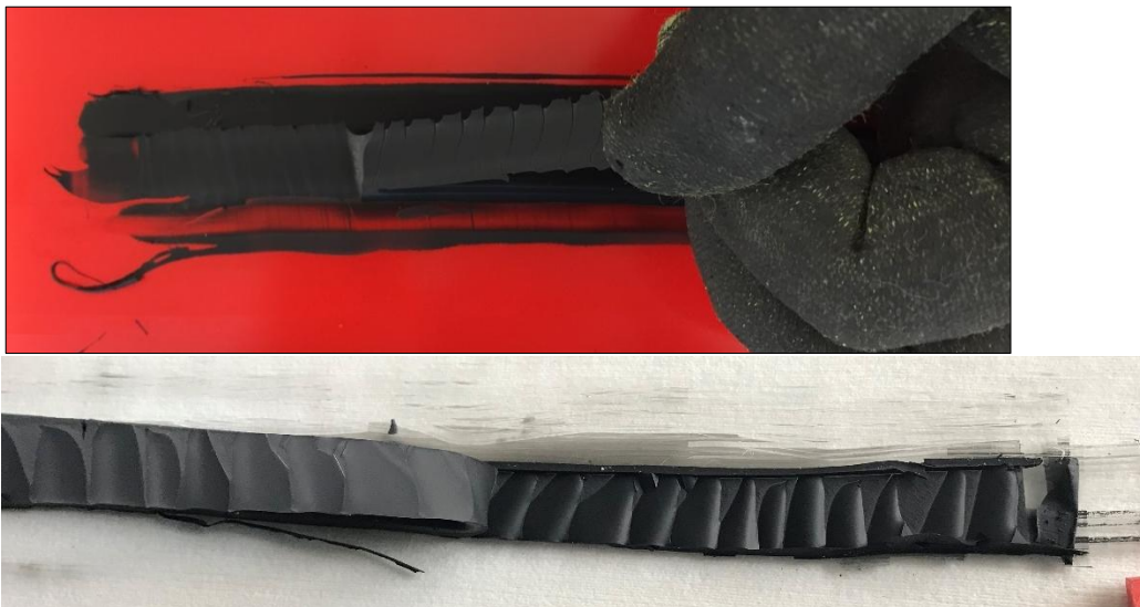
Figure 19: Peel adhesion test: pulling the bead apart; result: 100 % cohesive failure
