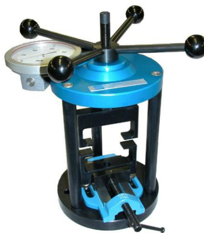
"Ban VEC" manual test bench with analog measurement (sold by GINGER CEBTP);
