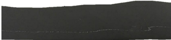
Figure 10: White stripe in material, inhomogeneous mixing
