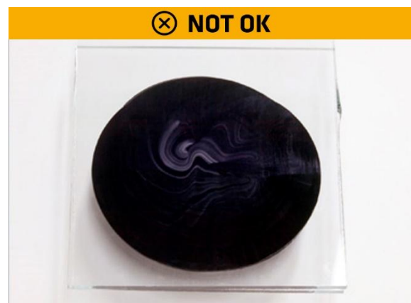
Figure 3: Negative test = inadequate mixing
